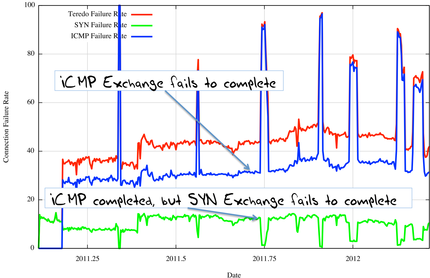
Teredo Connection Failures
